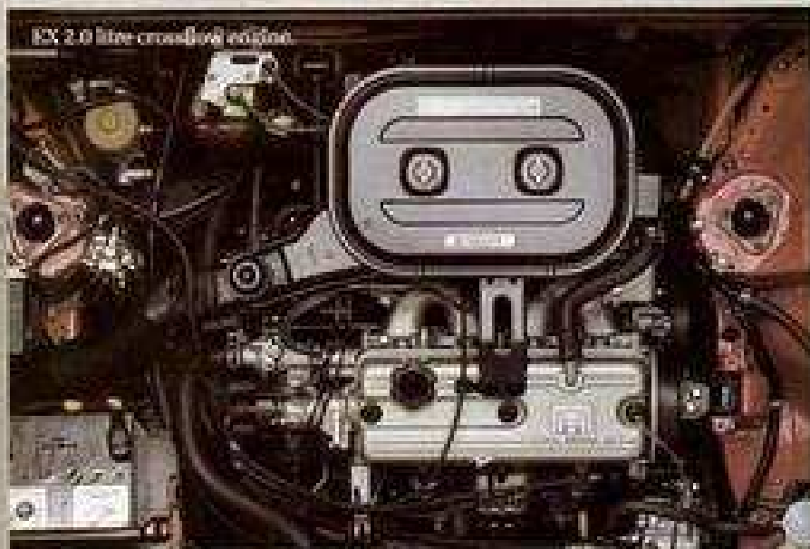
Crossflow cylinder head.
