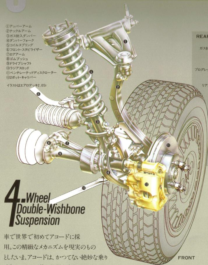
4-Wheel Double-Wishbone Suspension
