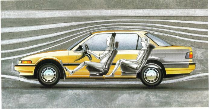
Exceptional aerodynamics have been achieved on the 1988 Accord models. A low hoodline is made possible by incorporating double wishbone front suspension. Also, flush-fitting body parts and retractable headlights further reduce wind resistance. Five passenger seating and ample trunk space contribute to the Accord's maximum space efficiency.
